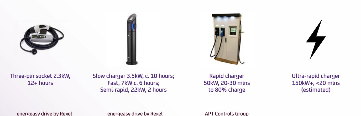
Figure 2: Types of charging technology and the average time needed to achieve full charge
